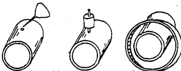
OIL FEED from automatic oiler, centre, is constant while machine operates. Only attention needed is occasional refilling of reservoir
