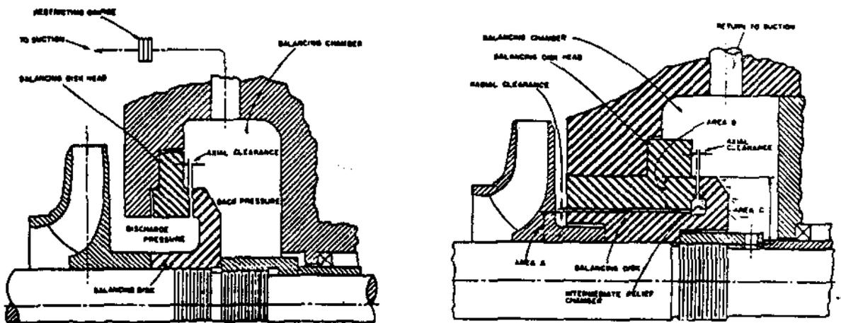
a. Simple balancing disc      b. Combination balancing disc and drum
