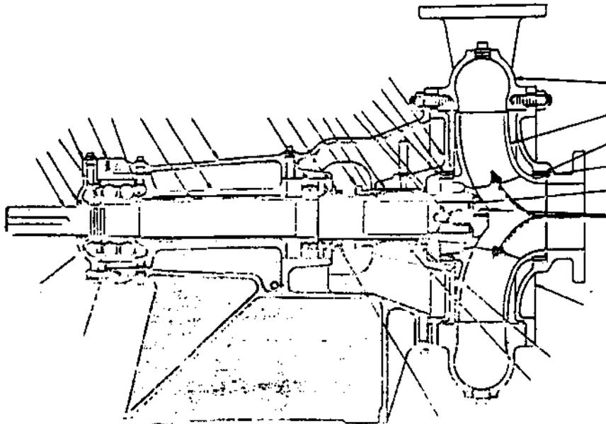
FIGURE 5: Single Suction Pump With 'Overhung' Impeller
