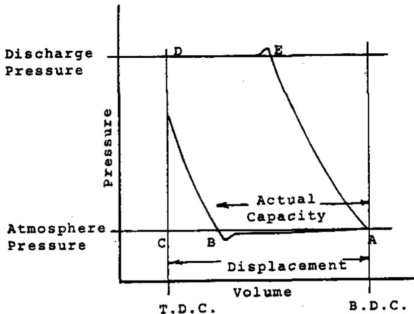
Effect of Cylinder Clearance on Volumetric Efficiency
