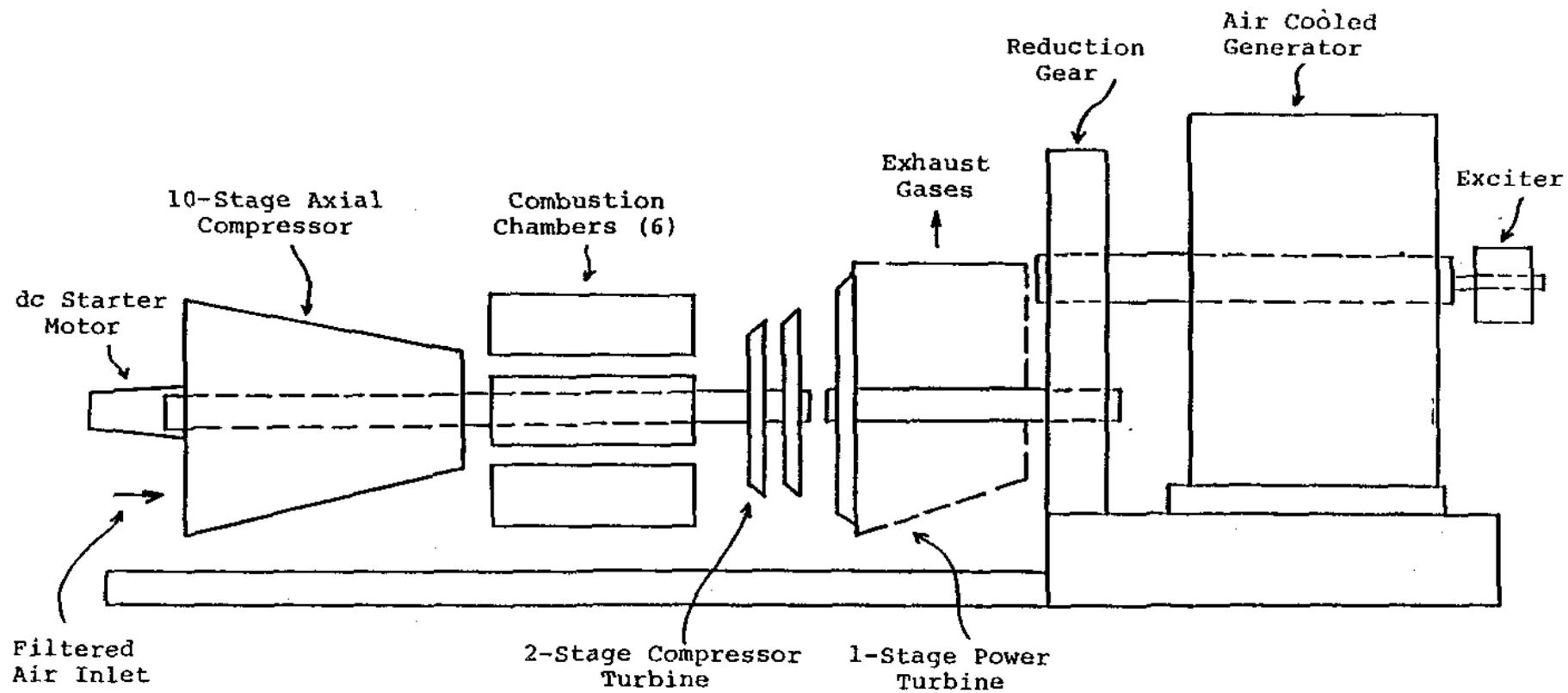
Gas Turbine Generator Basic Components
