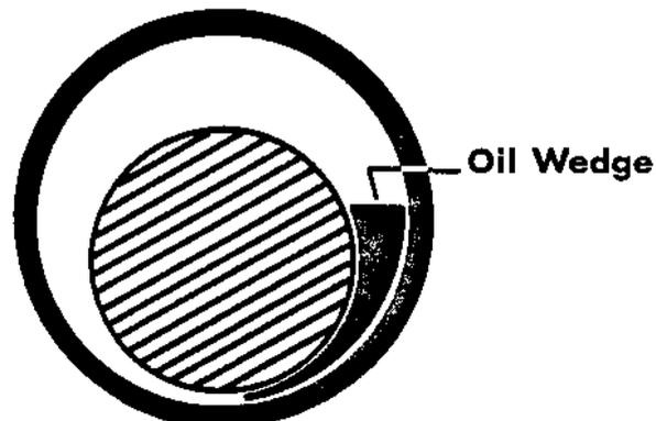
Since oil cannot be squeezed into a small volume, its pressure builds to separate the surfaces. To develop this oil wedge the following must be present:
