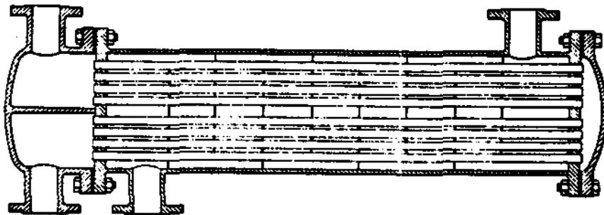
Shell and Tube Heat Exchanger
