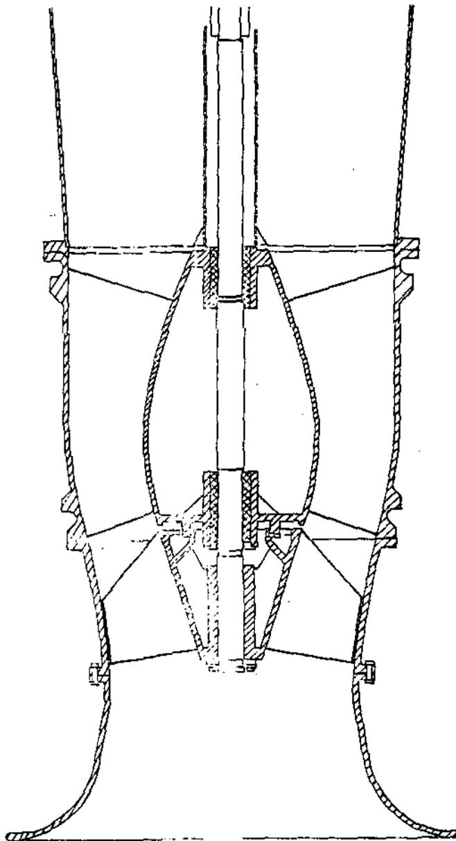
FIGURE 23: Pickering Condenser Circulating Water Pump
