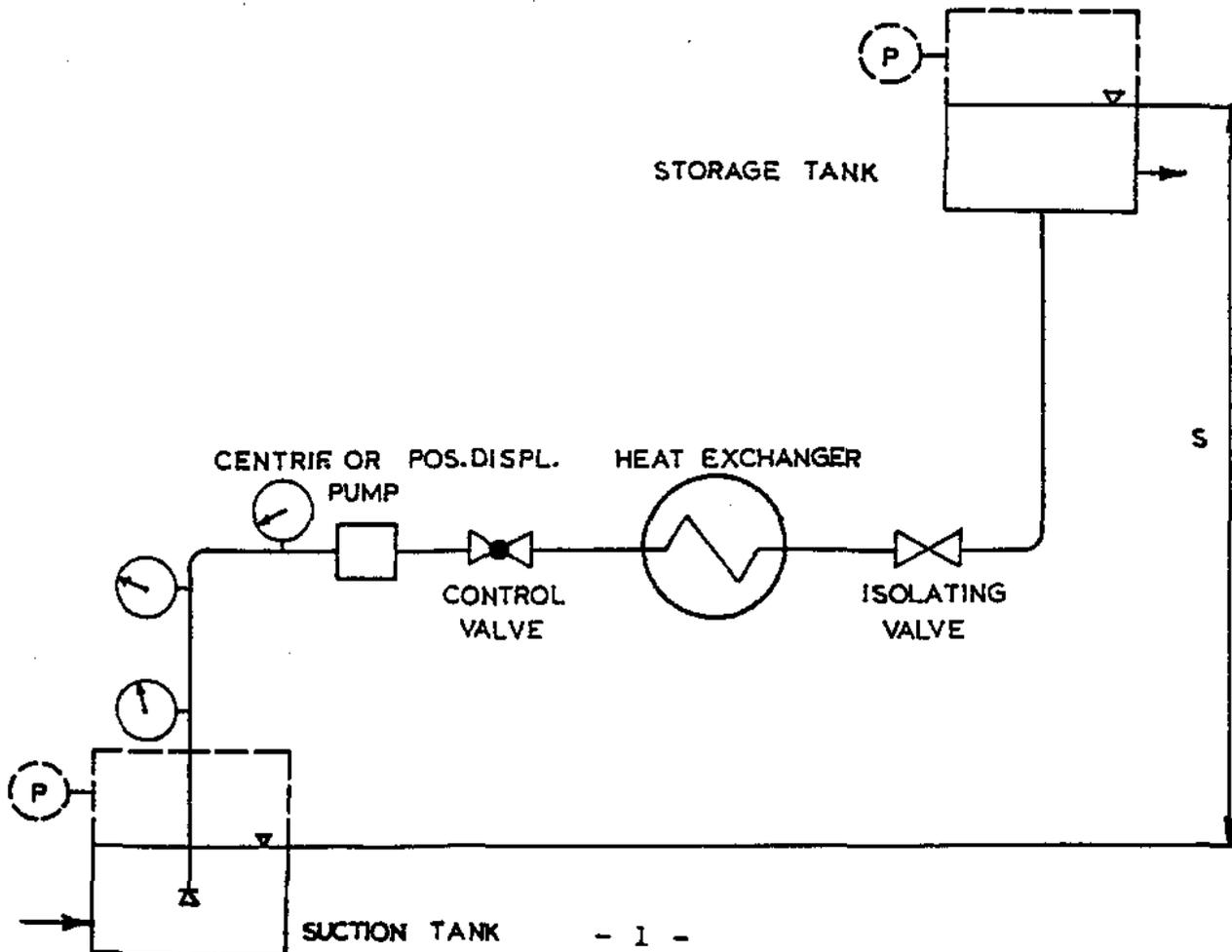
The pump works with so-called suction lift, because its centerline is above the suction tank. If it was below, we would talk about the suction head. The pump delivers the liquid through a control valve, a heat exchanger and an isolating valve into a storage tank where it is ready to be used further in the process.
