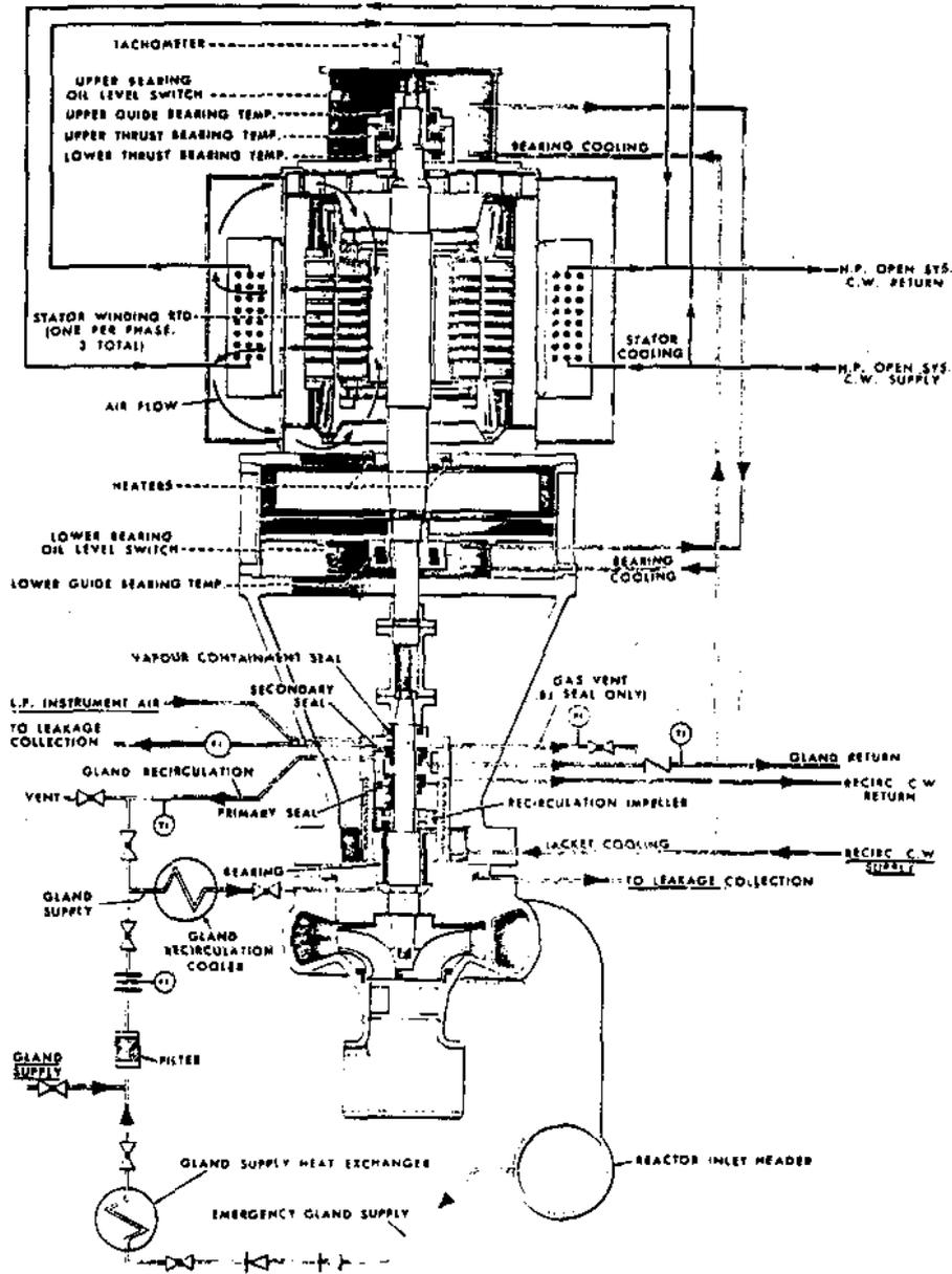
Pickering GS'A' Heat Transport Pump - Instrumentation and Auxiliary Circuits Schematic
