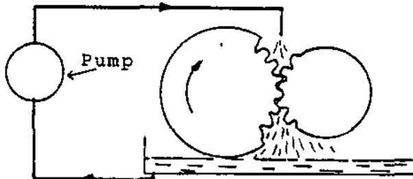
FORCE FEED applies oil direct to the pressure area. Oil conditioning unit can be installed in the feed line to extend life of the lubricant
