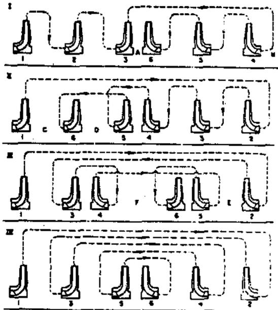
I. Joint A subject to three-stage pressure differential; one stuffing box under high pressure at B. II. Arrangement with two high-pressure joints, including four-stage pressure differential at C and two-stage differential at D. III. Joints E and F under two-stage pressure differential. IV. All running joints subject to only one-stage pressure differential.
