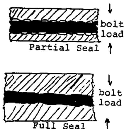
Gasket Must Be Capable of Flowing, When Under Bolt Load,
