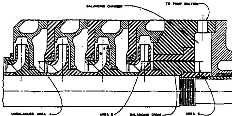
FIGURE 18: Balancing Drum
