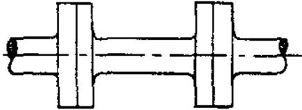
The main disadvantage of rigid couplings is that the alignment must be absolutely correct. If not then stresses can be created which fluctuate due to rotation and lead to fatigue problems.
