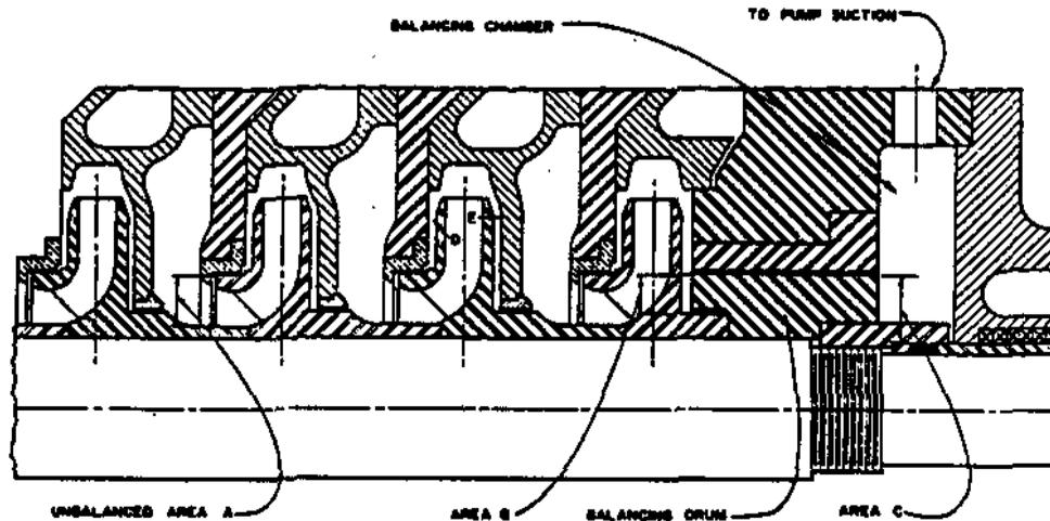
FIGURE 18: Balancing Drum
