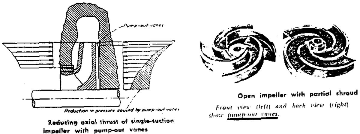
Reducing axial thrust of single-suction impeller with pump-out vanes
