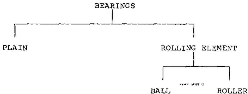
From the discussion on roles of bearings we mentioned that the primary role of a bearing is to support moving parts. Support means the bearing must be able to handle the different forces which act in the shaft.
