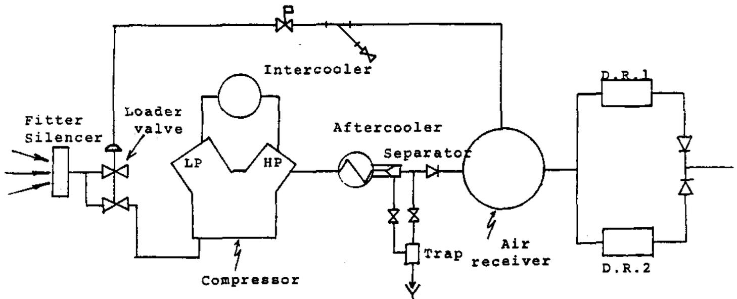
High Pressure Instrument Air Compressor
