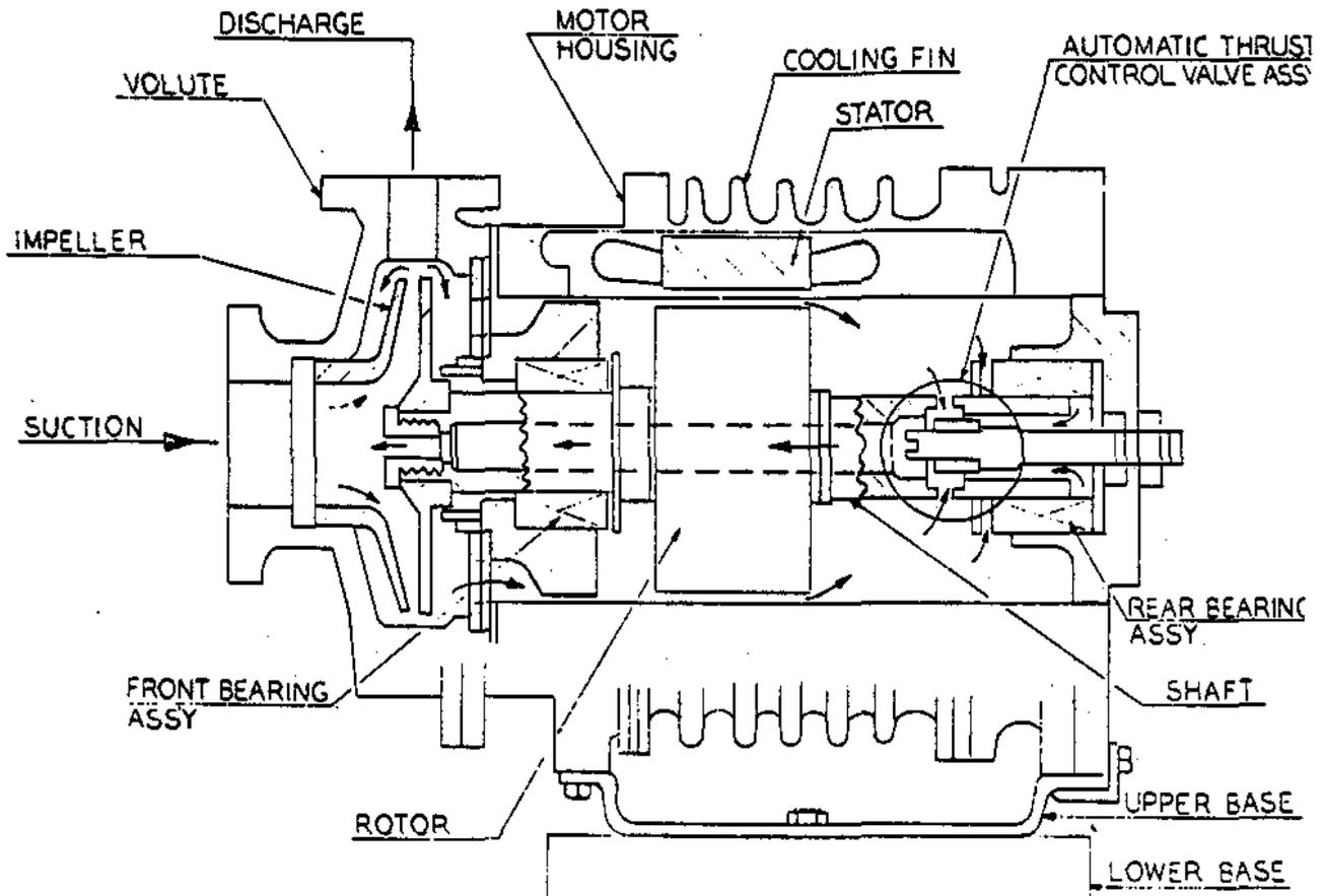
BHWP-Canned Rotor Centrifugal Pump With Internal Recirculation
