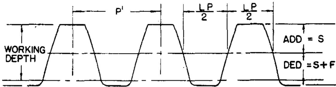
The Diametral Pitch (Pitch or P.) indicates the size of the tooth.
