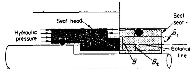
Partial balance achieved when head sealing face is lowered by means of a step cut in the sleeve. Hydraulic pressure acts against a portion of the total face area  $B$ . The factor of "per cent of balance" is created by distributing the area of  $B_1$  and  $B_2$  above and below the balance line respectively.
